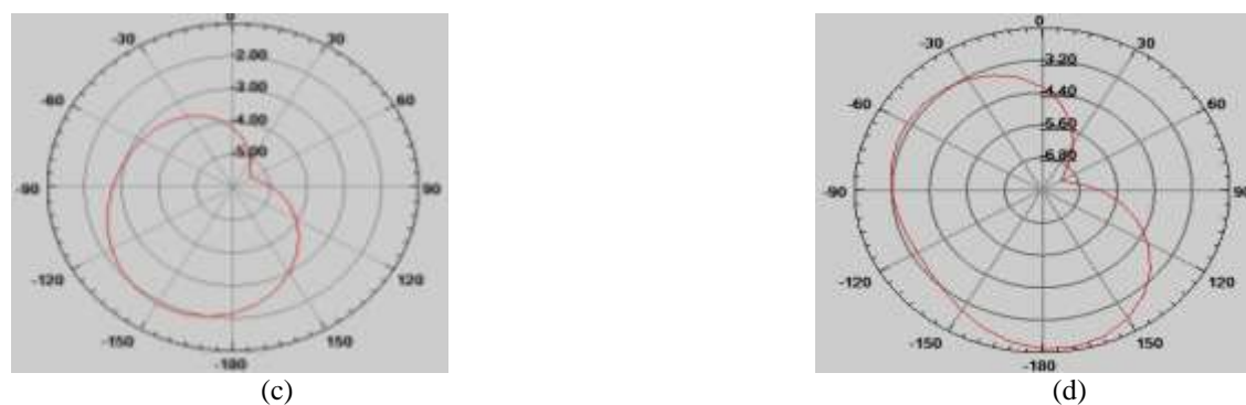
Figure 8: H Plane Radiation pattern at 6GHz frequency at (a) \phi = 0^\circ (b) \phi = 90^\circ (c) \phi = 180^\circ (d) \phi = 270^\circ
