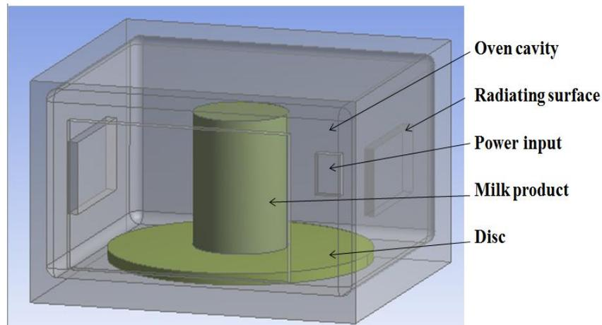
**Fig 1: Geometrical model of microwave oven**
