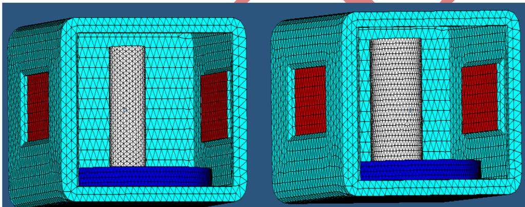
**Fig 3: Meshed diagram shows the location of microwave oven components**
