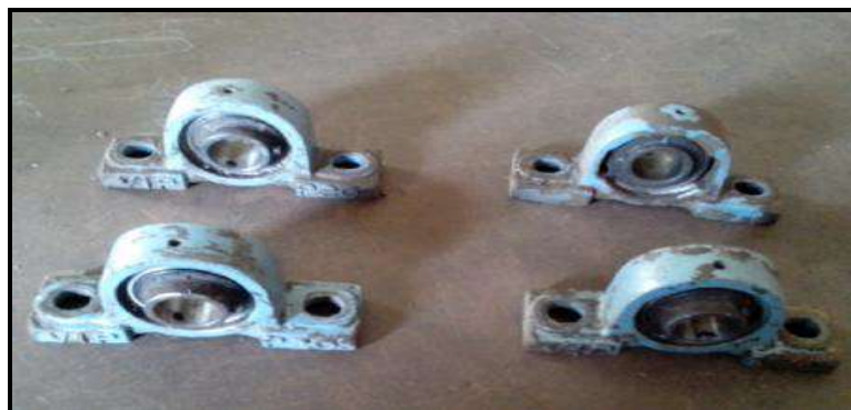
Fig(7) Plumber Block
