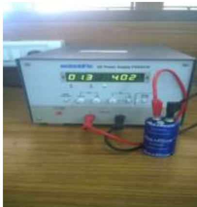
Figure 2. Setup for Charging of 100F, 2.7V and its Characteristics
