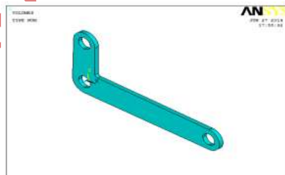
Fig.2-ANSYS Model of Bell Crank Lever.
