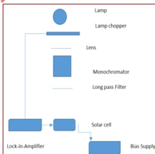
Fig. 3: Standard Arrangement of Spectral Response Meter
