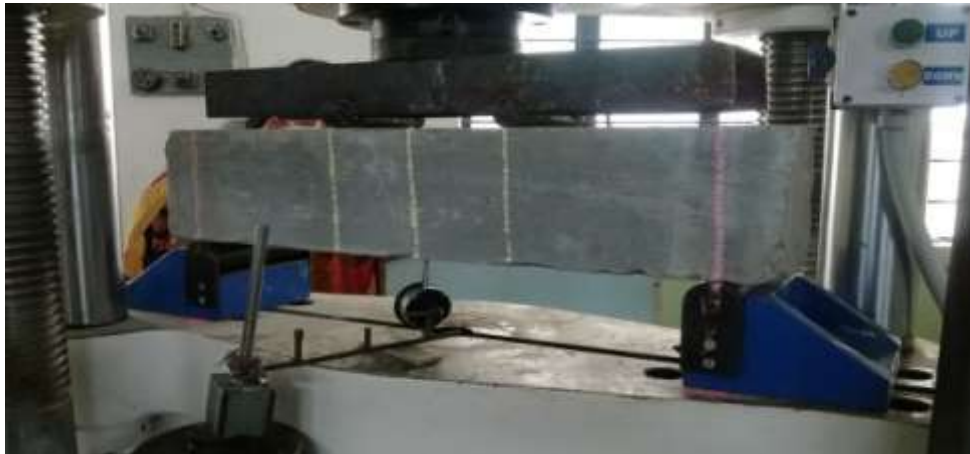
Fig.2: Experimental Setup for testing of beams
