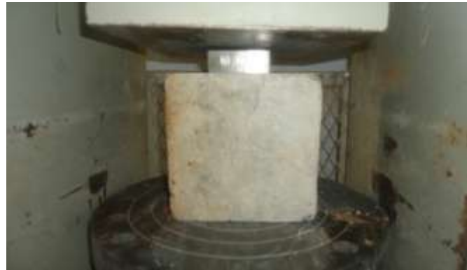
Fig. 6: Cubes testing for bearing strength using 67.1mm square plate
