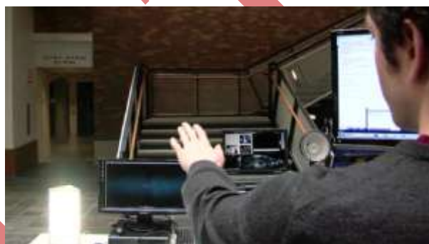
Figure 7: A student demonstrating how to turn on and off lights via gestures with a Kinect
