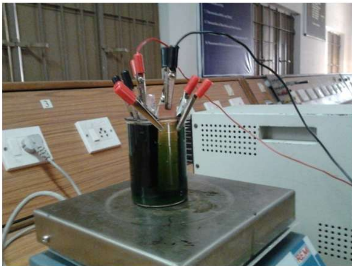
Figure 1: Experimental setup of electrodeposited CoNiP thin films
