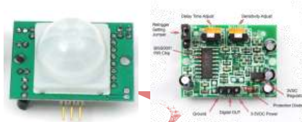
Figure 3.PIR Sensor Top and Bottom View [9]
