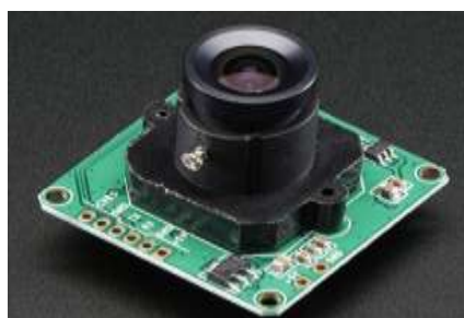
Figure 4 Serial Camera Module [10]
