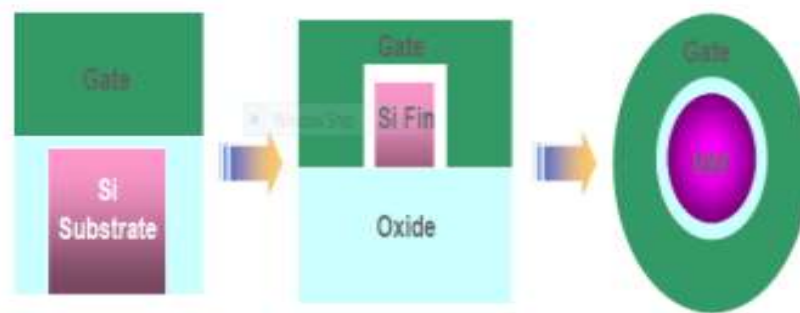
Fig 2: Progration of device structure from conventional single gate planar device to GAA structure
