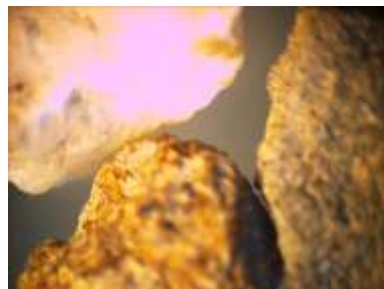
Fig. 8: Gravel 1, observed with stereomicroscope apparatus with magnification scale 8x. Carbonate aggregates, sandy material pieces with dimensions 2-4mm.
