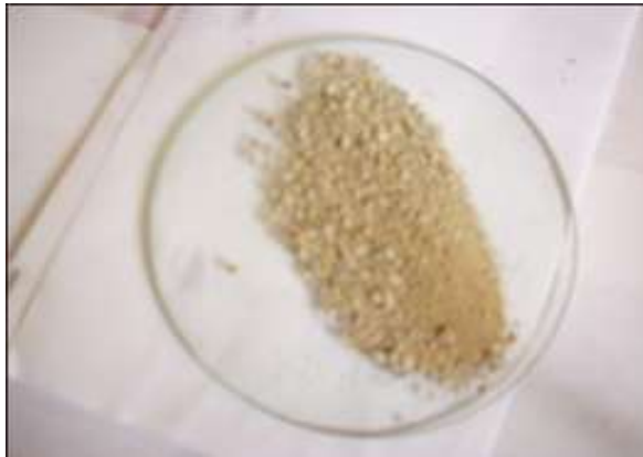
Fig. 1: Natural view of limestone sand. Fractioned, granular calcareous material with dimension ranging from hundredths to tenths of mm. Grain size is 1-3 mm.
