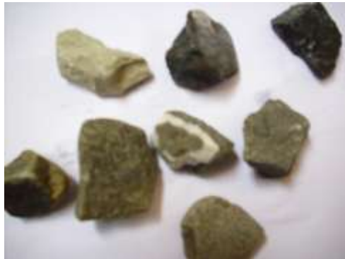
Fig.16: Gravel 2: Natural view (32.5-45 mm) grain size. Basalt pieces with green black color, sandy pieces with yellow-darkness color, alkaline volcanic rocks pieces with green color, small microcrystalline of calcite secondary ( \text{CaCO}_3 ) with white color and dimensions 2-5mm.
