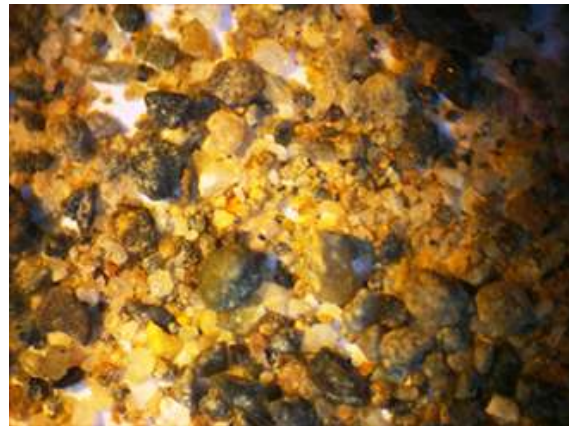
Fig. 4: River sand, observed with stereomicroscope apparatus, with aluminosilicate magnification scale 8x. Chloride aggregates-grains, olivine, pyroxene, olivine – quartz and calcite.
