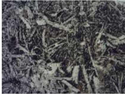
Fig. 17: Gravel 2, pieces, basaltic texture with darkness to black color composed from plagioclase rods with size up to 0.2mm, chlorite cement with opac minerals (metallic, such as magnetite, pyrite etc.) observed with polarized light microscope with magnification 40x.
