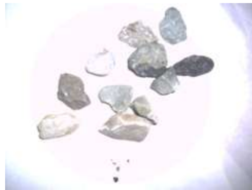
Fig. 10: Gravel 2 (1-2 cm), natural view. Fractioned sandy material represented with beige-darkness color, while calcareous material is represented with white-grey color., Siliceous-chloride base volcanic rocks represented with green to darkness color.
