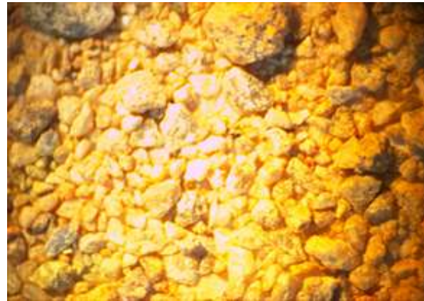
Fig. 2: Limestone sand observed with stereomicroscope apparatus with magnification 8 x. Calcareous granular aggregate represented by beige – yellow colour.
