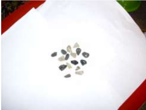
Fig. 9: Gravel 1, 8-14 mm, natural view. Sandy material made of fractioned aggregates. Basalt is represented by darkness pieces and calcareous material is represented by white-grey pieces.
