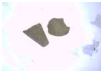
Fig. 20: Natural view of sample 32.5-40 mm grain size. Fractioned sand pieces, shaped plate with gray to dark beige color.
