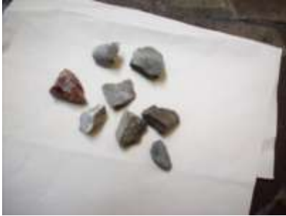
Fig. 11: Gravel 2, natural view (12.5-20 mm). Sandy aggregate pieces, chloride volcanic rocks, calcites, while red siliceous pieces are very rare (mainly formed by iron hydroxides).
