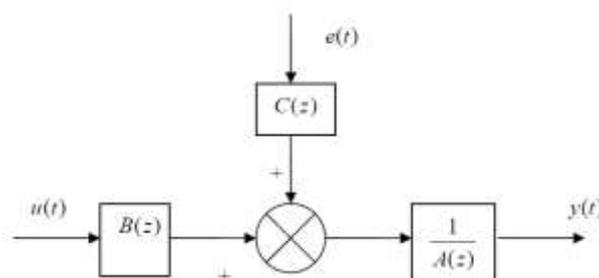
Fig 6 ARMAX Structure
