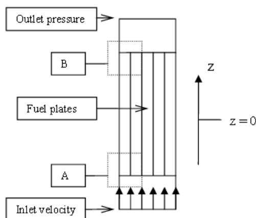
**Fig 3 Boundary conditions on Fuel Assembly**
