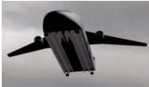
Fig. 1: An Aircraft with Pulse Ejector Thrust Augmenter (PETA) Modules
