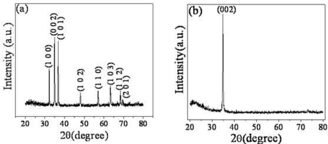
**Fig. 1: Xrd Pattern Of ZnO Thin Films Grown By Sol-Gel Spin Coating Method On Quartz Substrates Using Various Sol Concentrations (A) 0.6M And (B) 0.4M**
