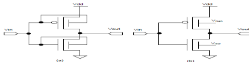
Fig.3.5 FinFET Inverter (a) Shorted gate & (b) Low power gate
