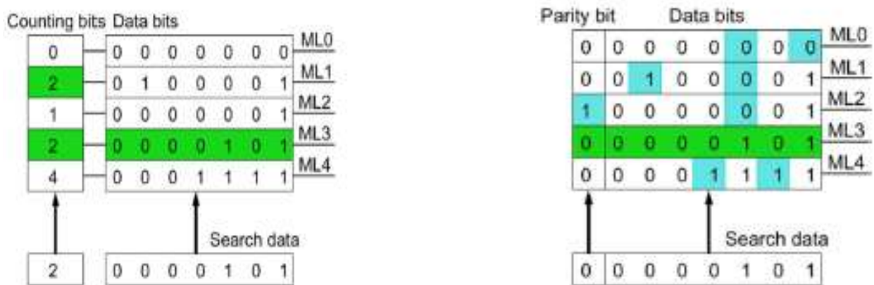
Fig 4.1 a) Conceptual View of Pre-computation based CAM design b) Conceptual View of Parity based CAM design
