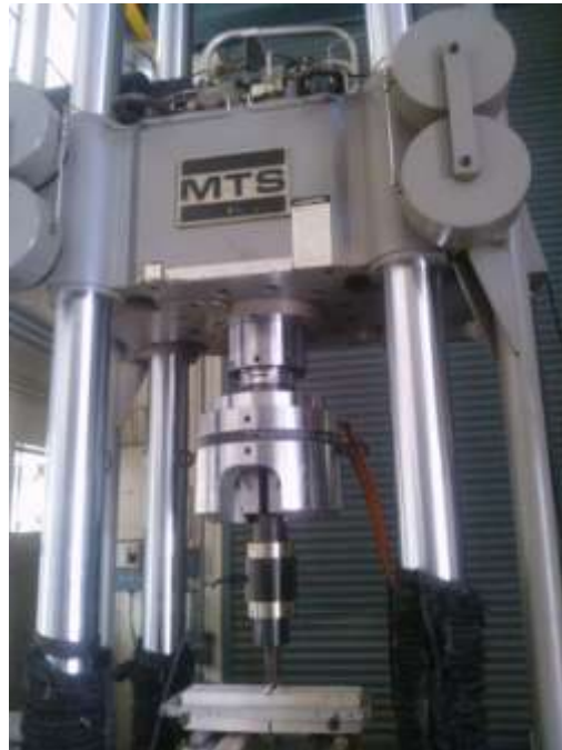
Figure 1 : Three point bending test on notched prisms
