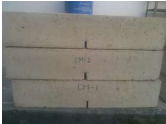
c) Crack formed in specimens without fibres
