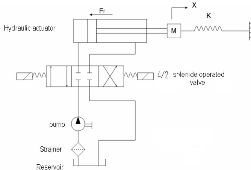
**Figure1: The Hydraulic System and Hydraulic Actuator**
