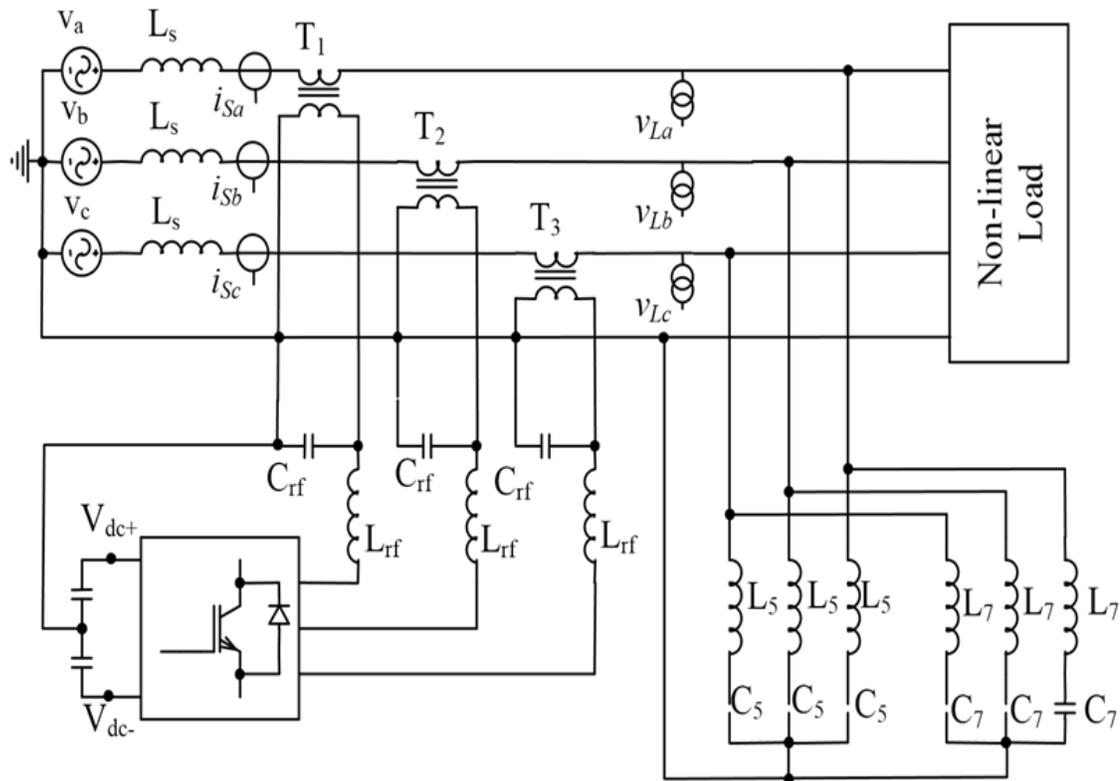
**Figure 1. Series active filter and shunt passive filter topology**
