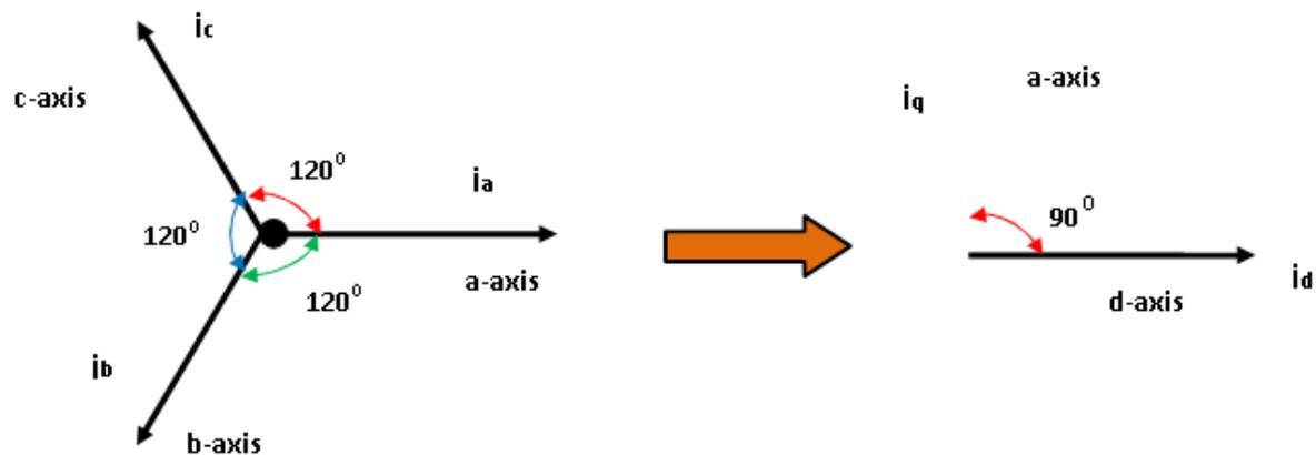
**Figure 3. Transformation from the phase reference system (abc) to the (0αβ) system.**
