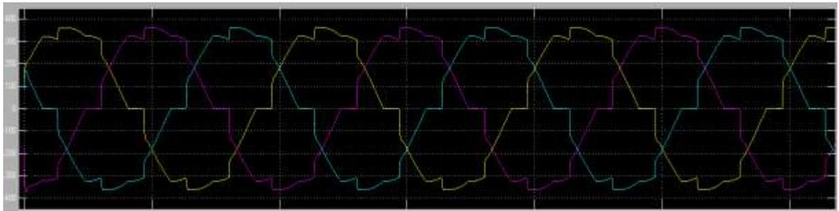
Figure-5 Waveforms of source voltage without filters
