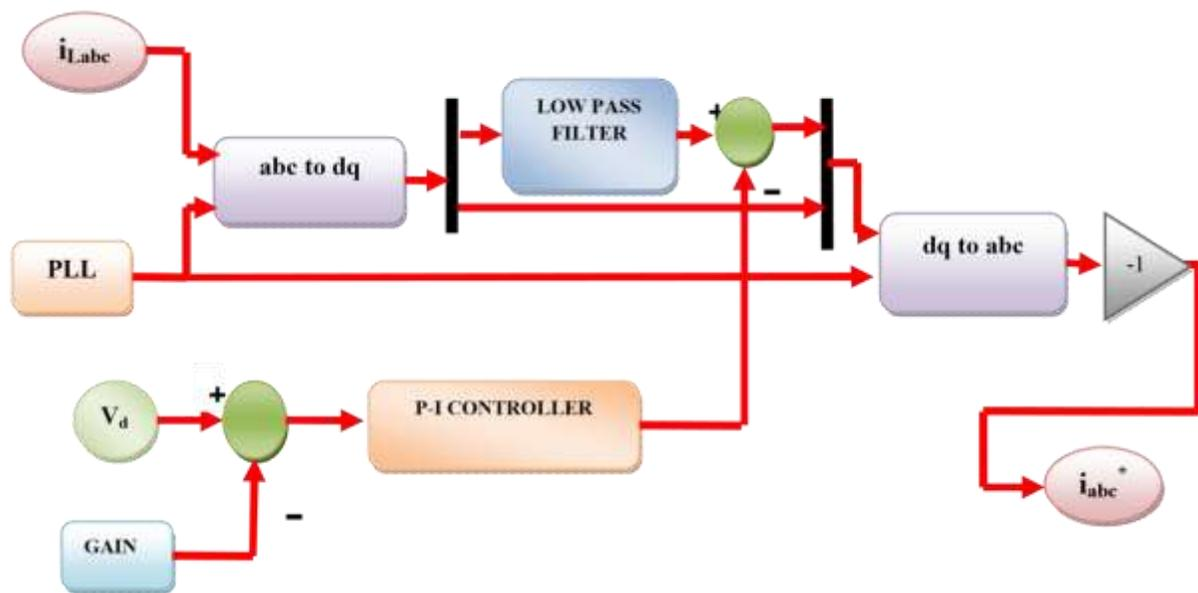
**Figure 2.Synchronous d-q reference frame based compensation algorithm**
