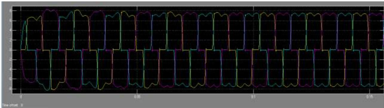
**Figure 8 Waveforms of load current with hybrid filter**
