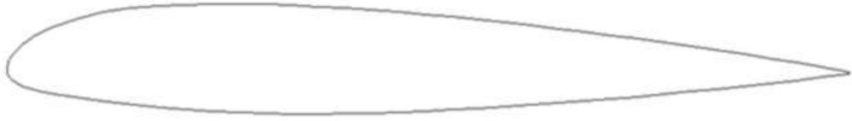
**Fig 3: NACA 23012 Airfoil**
