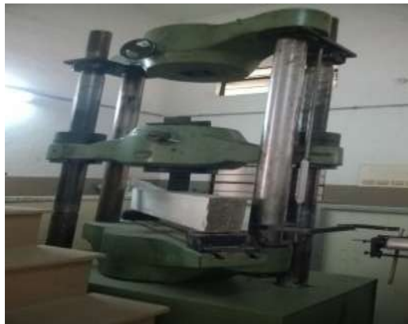
Figure 4: UTM used for testing all specimen.
