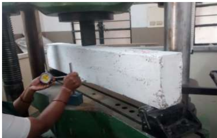
Figure 2. Experimental setup for testing of RC beam under three point bending
