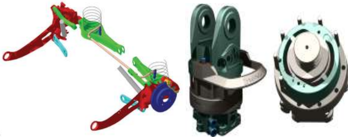
Figure.1.MBS simulation model of vehicle suspension and CAD model of hydraulic rotator.
