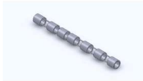
Fig.6 Isometric View of the Pre Detonator with Shchelkin Spiral
