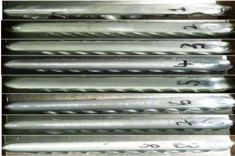
Fig 3. Visual inspection of welds.
