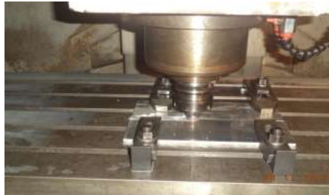
Fig 2. FSW experimental setup
