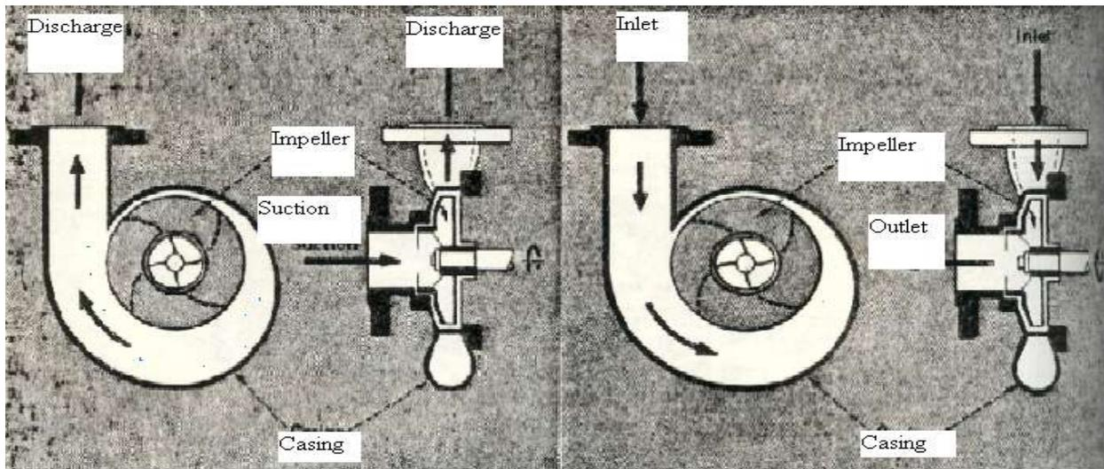
**Fig.1: Pump in pumping and turbine mode**
