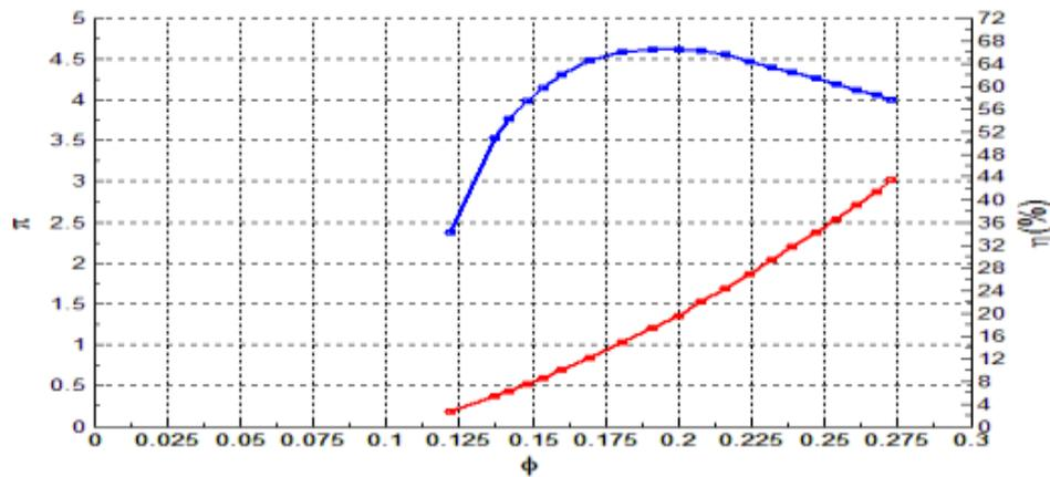
**Figure: 3 Power number and efficiency for 38.47 rpm PAT at 1100 rpm speed**
