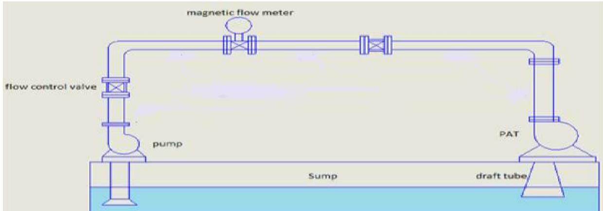
**Figure : 2 Layout of test rig**
