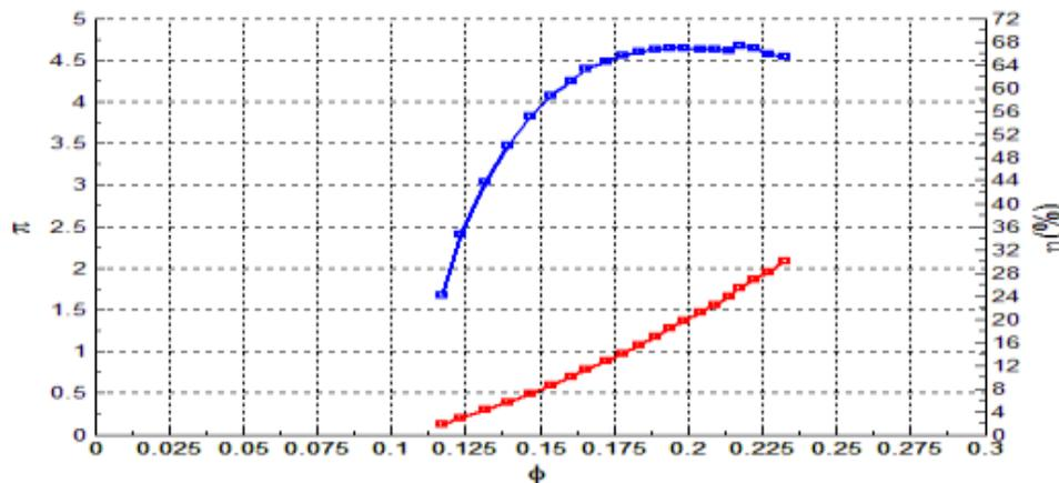
**Figure 4: Power number and efficiency for 38.47 rpm PAT at 1300 rpm speed**
