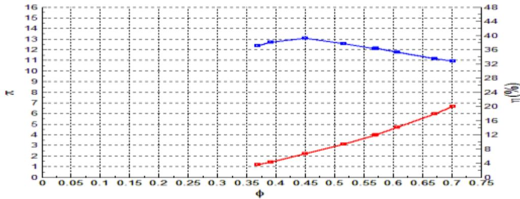
**Figure: 5 Head number and efficiency for 53.83 rpm PAT at 700 rpm speed**
