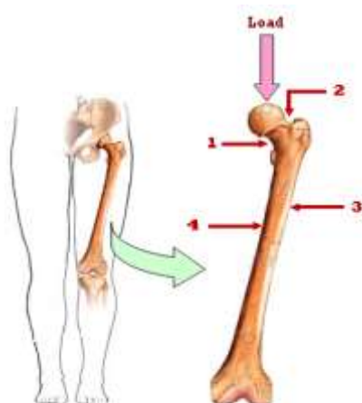
Fig.3: Positions Of Strain Gauges
