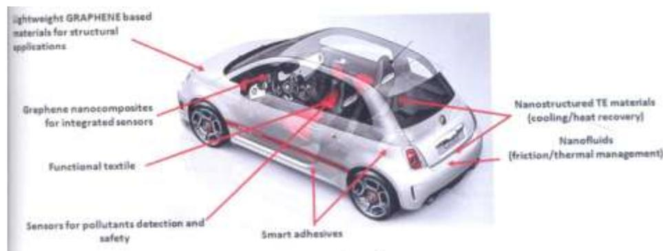
**Fig. 5: Future Potential Application of Graphene in Automobiles**
