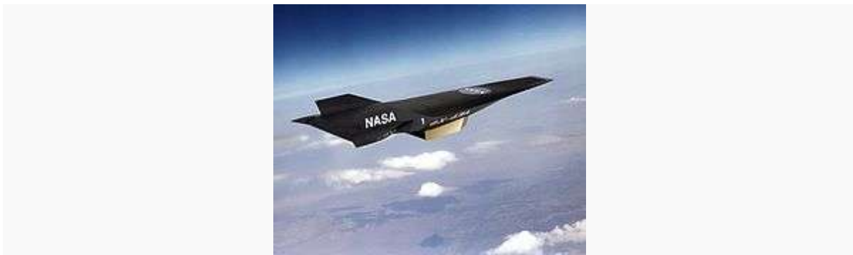
Fig.1 NASA X-43with scramjet attached to the underside
