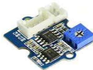
Fig 5 Piezo Electric Vibration Sensor.
