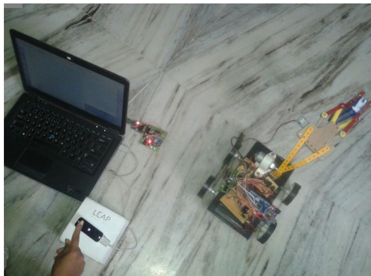
Figure 7 Robotic Arm Grasping the Object According to the Hand Gestures Given by the User
