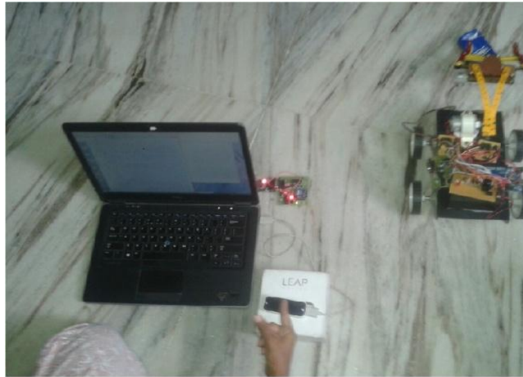
Figure 8 Robotic Arm Releasing the Object According to the Hand Gestures Given by the User
