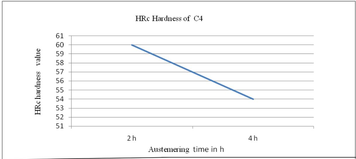
**Fig.6 Variation of Bulk Hardness with Austempering Time of C4**
