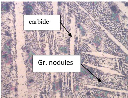
Fig. 4(a)C4-4hr-200x shows carbides and Ausferrite.
