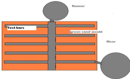
**Fig.1(a) Sample Casting Green Sand Mould.**
