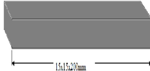
**Fig.1(b) Sample Test Bars.**
