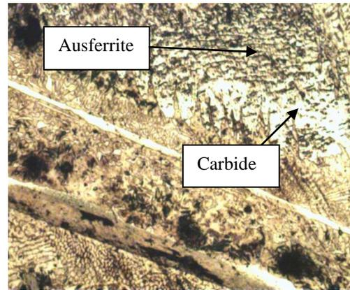
Fig.3(b) C4-400<sup>0</sup>c-2hr-200x shows ausferrite.
