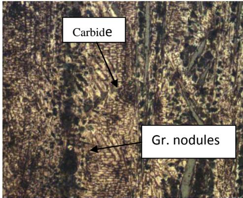
Fig. 3(a) C4-400<sup>0</sup>c-2hr-200x shows carbides and Graphite nodules
