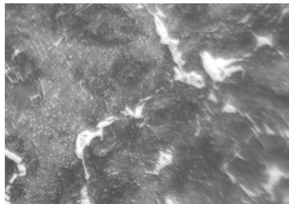
Fig.5 Show Microstructure of Austenitized at 900<sup>0</sup>C Austempered at400<sup>0</sup>C-2h at 500X.
