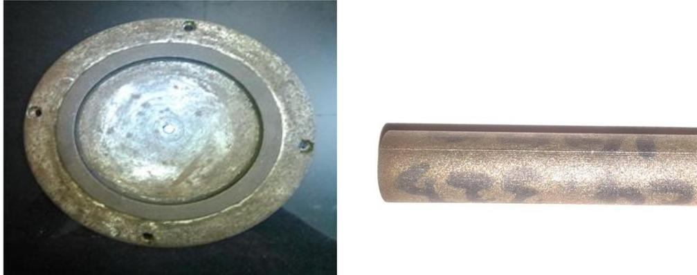
**Fig.2 Show the Wear Samples of CADI 8mm Diameter and Counter Face Wear Base Plate.**
