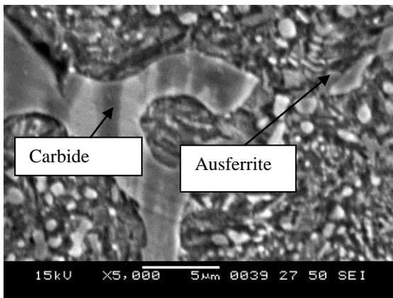
Fig. 9(a)Show SEM image 900<sup>0</sup>c 400<sup>0</sup>c 2h at 5000X.
