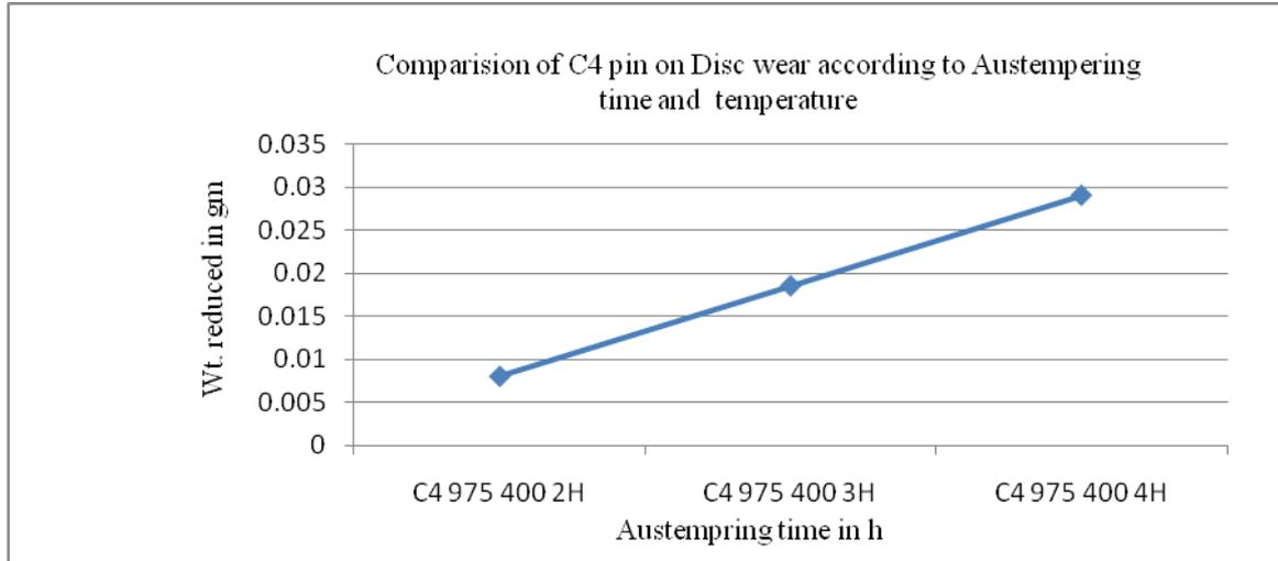
Fig 7.wt. Reduced in gm Vs. austempering time in h.
