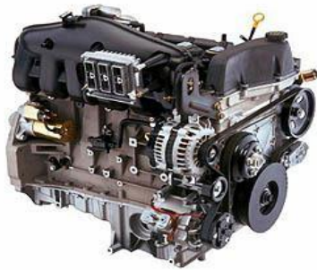
Fig (i) Straight/ Inline Engines
