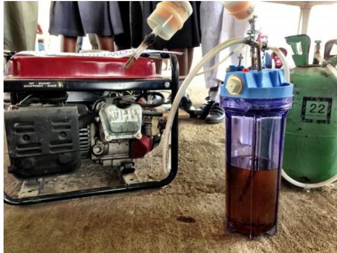
Fig 5: A Urine Powered Generator
