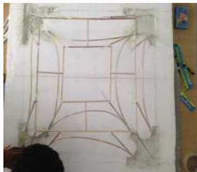
Figure 10. Top view of base foundation using plaster of paris
