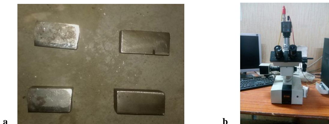
Fig.5. Microstructure Testing (a) Samples for Microstructure Test (b) Optical Microscope
