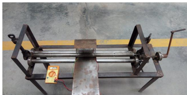
Fig.11. Experimental Set up for testing on three roller bending machine.
