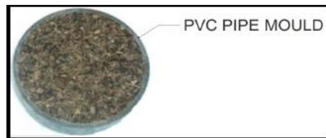
Fig.1 Mould used for Specimen Casting
