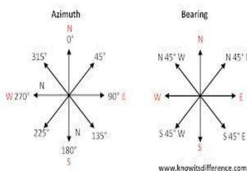
**Azimuth and bearing**
