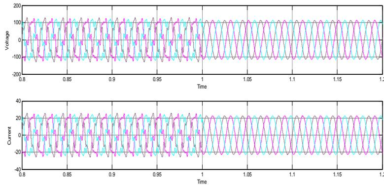
Fig 9 : Simulation waveforms when IPQC is not employed and after breaker applied and IPQC employed in case-2
