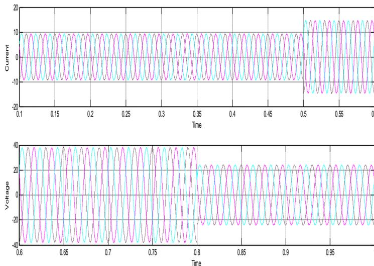
Fig 8 :Current and voltage waveforms of the primary winding when  $\alpha$  suddenly changes from 0.1 to 0.6 and 0.6 to 1
