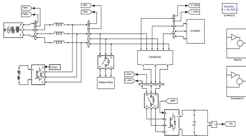
Fig 7: Simulation circuit to verify principle of variable reactor, harmonic isolation
