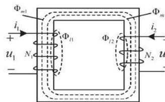
Fig 2: Magnetically Coupled Circuit of the Transformer
