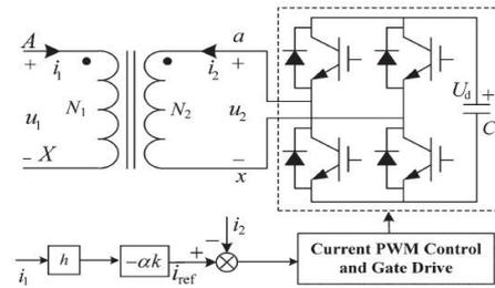
Fig 1: System Configuration of the Novel Variable Reactor
