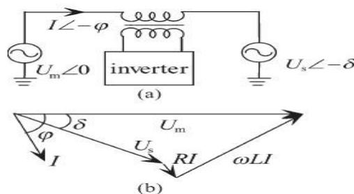
Fig 6: Power Flow Control Principle and Its Vector Diagram
