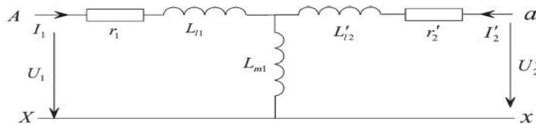
Fig 3: Equivalent T-Circuit of the Transformer
