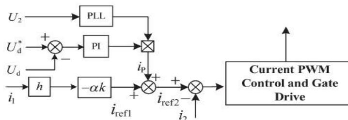
Fig 4: DC Link Voltage Control Schemati
