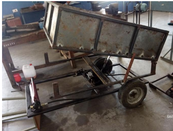
Fig: Modern Three Way Dumping Trolley Layout
