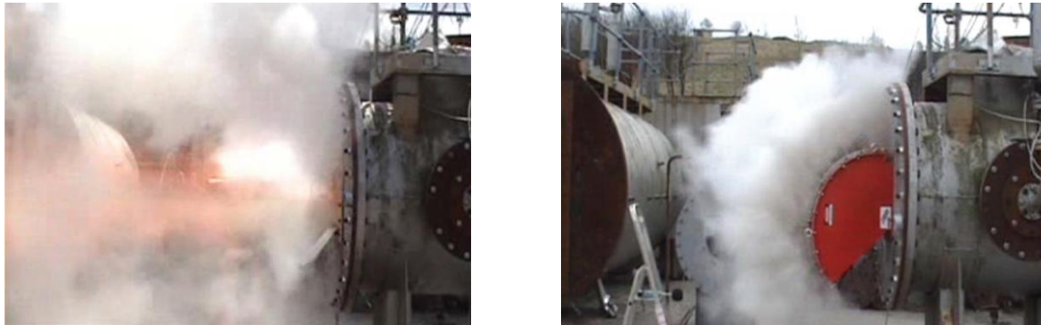
Fig. 4.5 Vented explosion test with a flameless venting device.
