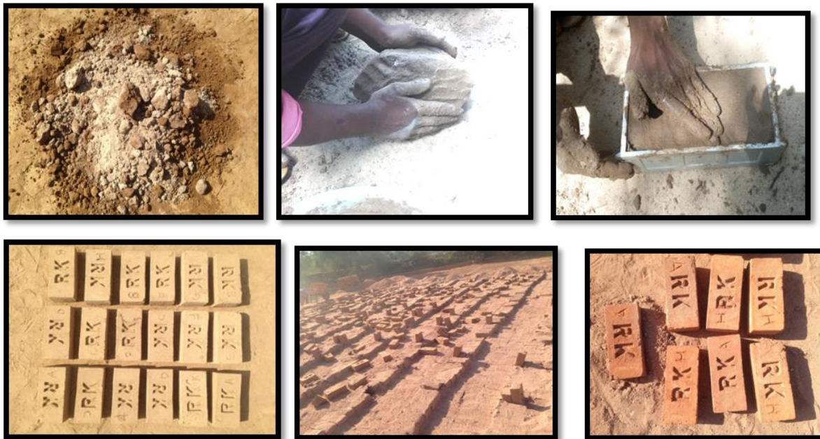
Fig. 1 procedure of making bricks
