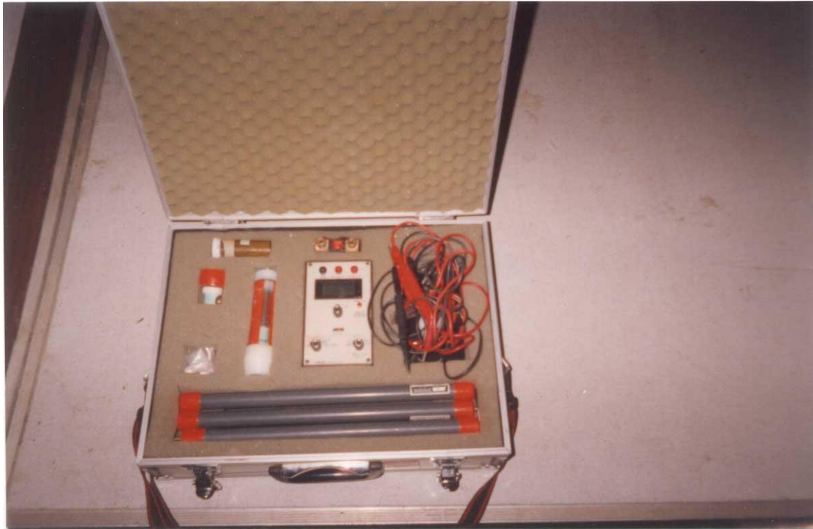
Figure 3 (a) Half-cell potentiometer at a glance
