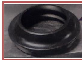
The component or part due to which the defect occurs is termed as DUST SEAL. Its main function is to protect the oil seal from dust contamination so it must be firmly pressed with the surface of the outer tube.
