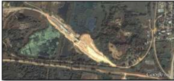
Snapshot after embankment failure after additional widening of the base
