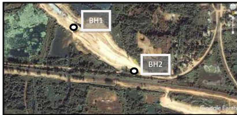
Fig 4.1 Borehole Location Map
