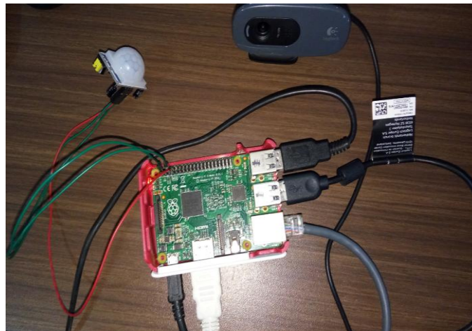
PIR Sensor and webcam are interfaced with Raspberry pi
