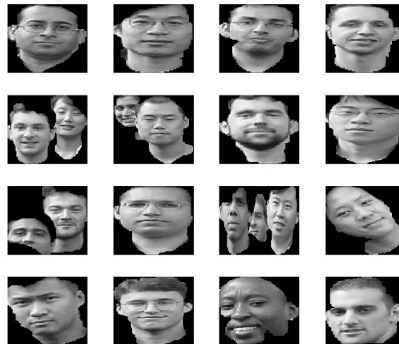
Figure 3.2. The output of connected region analysis for training image 1.
