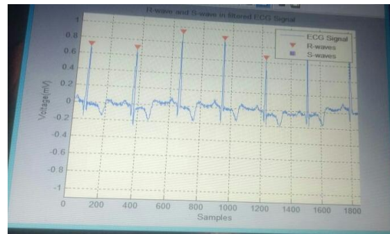
4.4 R-Wave and S-wave in filtered ECG signal
